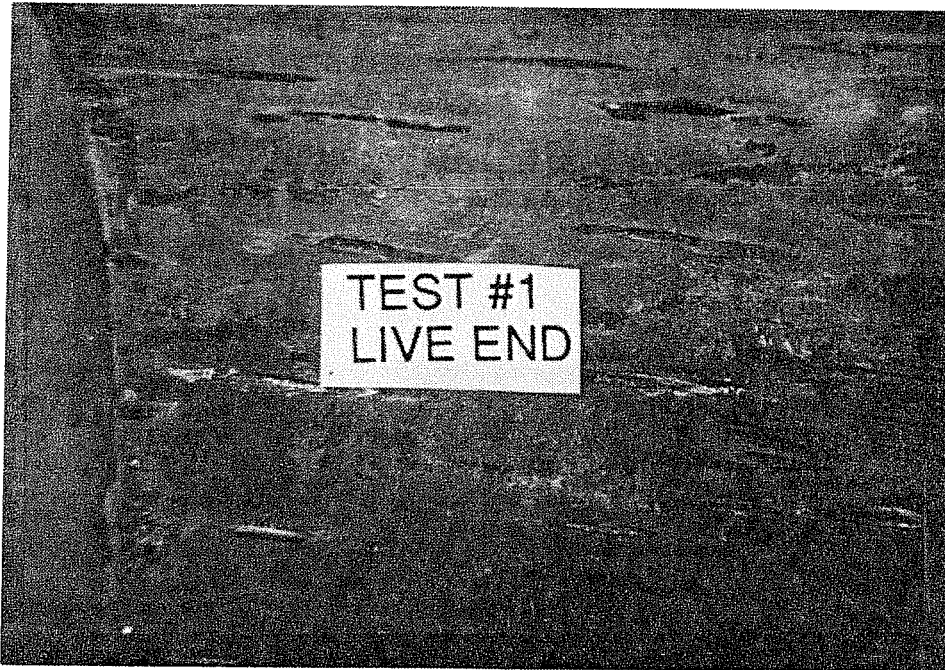
Figure 4.9 Evidence of fretting damage to inner section of the deviator duct in Test #1.
